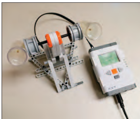
Clinostat made using Lego® Mindstorms® NXT robotic system. Photo by Travis Kelleher © Baylor College of Medicine.
