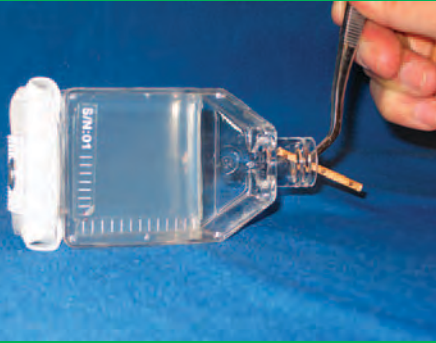
Demonstration of how an astronaut on the ISS will insert a balsa wood strip with attached seeds into a prepared flask. Photo courtesy of BioServe Space Technologies.
